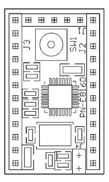
The dsEDGE E8160 is a low cost and flexible microcontroller solution, based on the Microchip 18LF2510 8-bit Microcontroller. The E8160 is designed for use at the application edge and can be placed virtually anywhere to provide low power, local processing for a variety of tasks.
